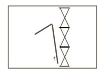
• Fold magnetic bar into 3, ensuring the magnets aren't touching eachother.
