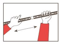
• To dismantle the frame, push on middle hub at back of frame while pulling on corresponding front hub. Nomadic Instand will sink to the floor. Handle frame at the hubs.
