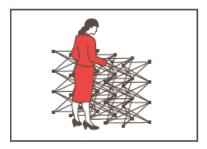
• Press front and back hubs in the centre of the frame until it locks into position (front and back hubs do not meet – but you will feel it lock into place).
