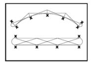
• Place the frame in the correct place before moving onto attaching the graphic panels, as the frame becomes difficult to move once the graphics panels are attached.
